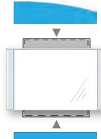
1/8" Thick Acrylic or Wood Laminate Accent Shape Attaches to the Aluminum Connector, Flush with the Top (and / or Bottom) of the Arris Frame.
