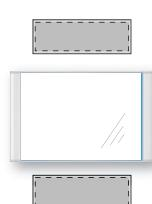
.040" Aluminum Connector with Pre-Applied Adhesive Attaches Securely to the Back Side of a Standard Arris Frame.
